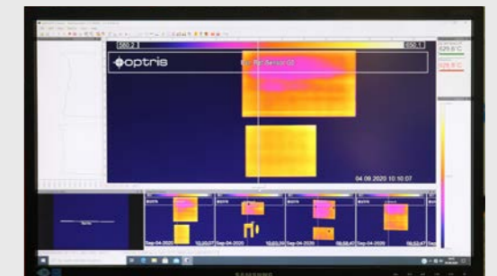
Monitoring temperatures of glass sheets
