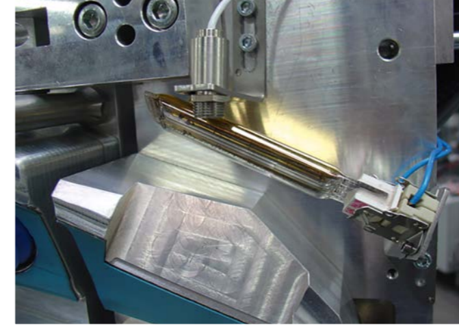
Infrared temperature measurement in packaging machines
