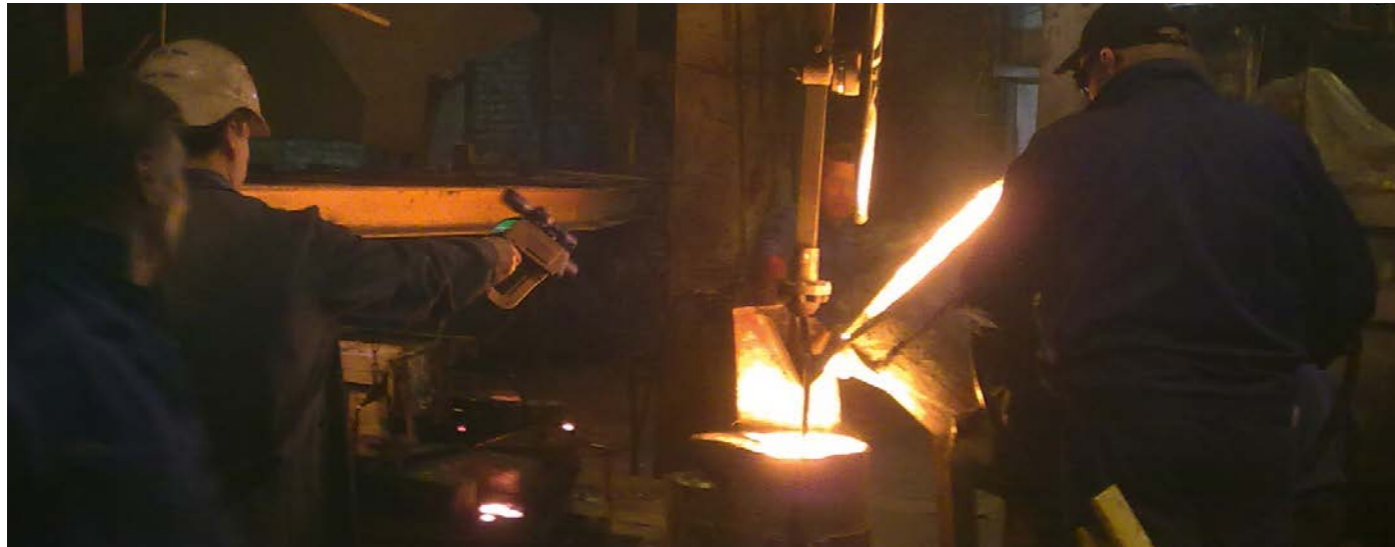
Detailed infrared temperature measurement on a melt in the casting plant with the P20 05M.
