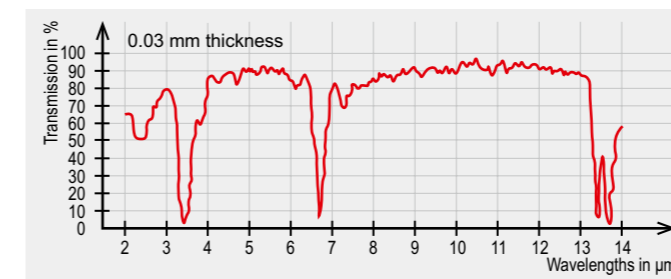
Spectral transmissivity of plastic films made from polyethylene
