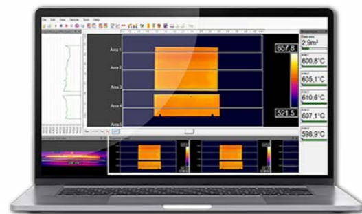
Monitoring temperatures of glass sheets with PIX Connect software
