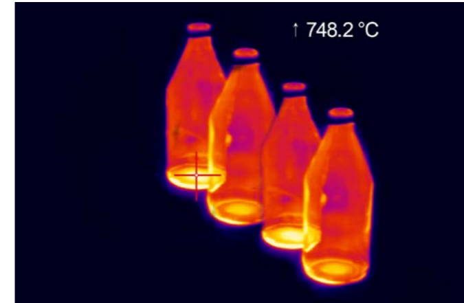
Hot spot detection in glass bottle production
