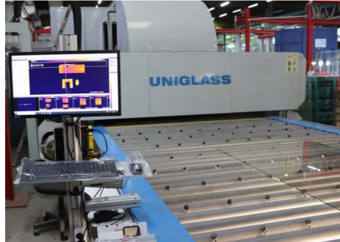
Temperature monitoring of glass sheets in a tempering machine
