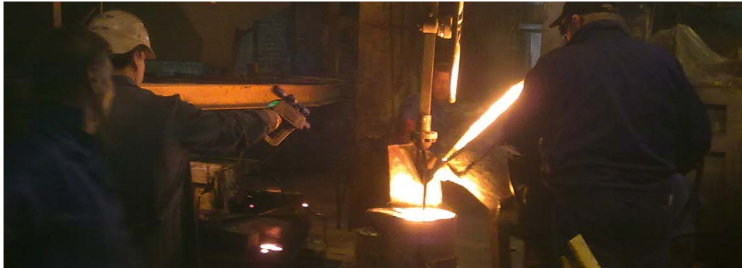
Detailed infrared temperature measurement on a melt in the casting plant with P20 05M.
