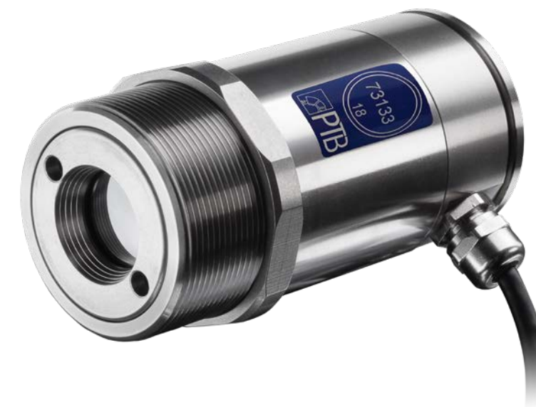
transfer standard radiation thermometer CT-PTB
