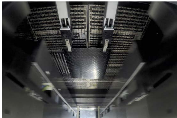
CT LT - Measuring head with laminar air purge device in a thermoforming machine
