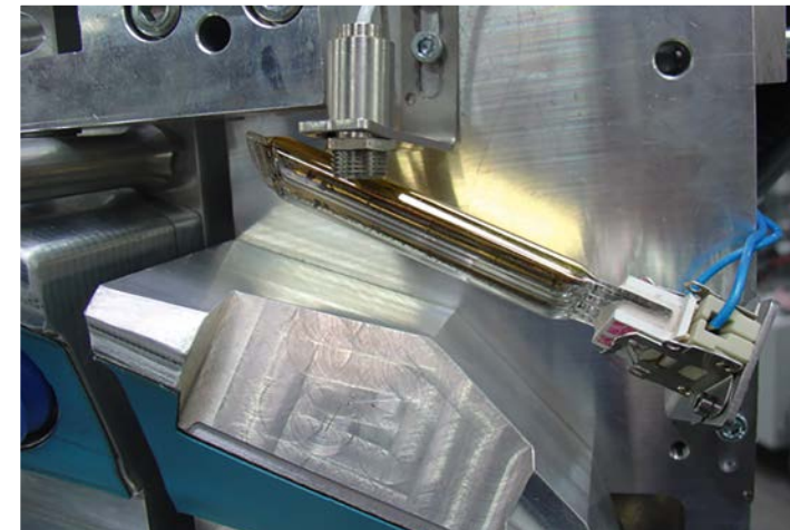
Infrared temperature measurement in packaging machines
