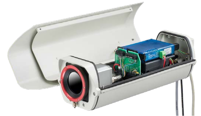
Outdoor protection housing with infrared camera of the PI series
