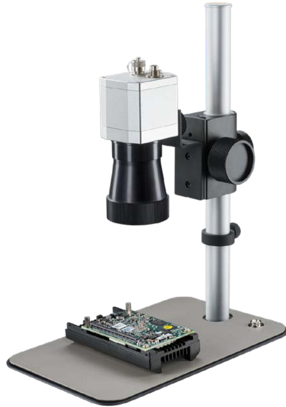
Microscope optics PI 640i for the inspection of PCBs
