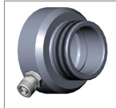
Figure 7: Air purge collar [ACCTLAP] Hose connection: 6x8 mm Thread (fitting): G 1/8 inch
