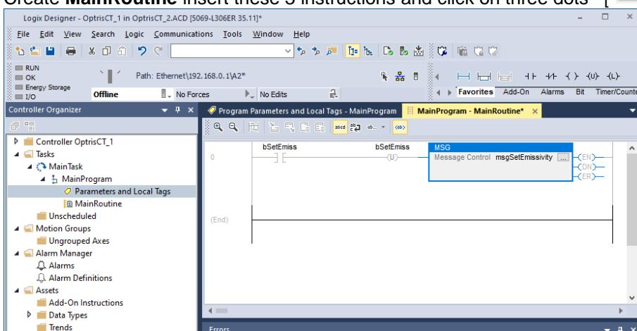
Set the configuration values according to **Table 3**, set the communication path to OptrisCT, and click on **OK**. Download the project to the PLC and start the PLC program in **Run Mode**.
