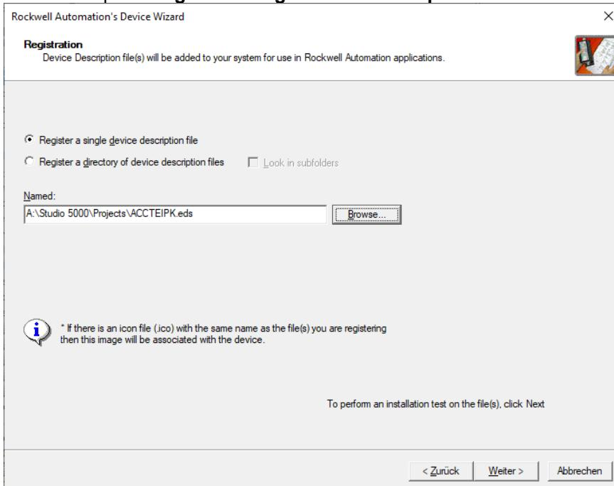
Click **next** until the message appears that the installation is completed and close the software "Rockwell Automation – Device Description File Installation Tool".
